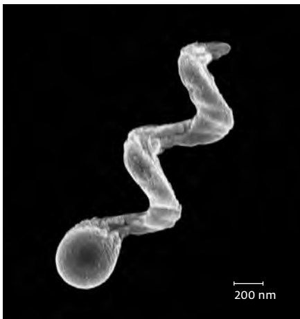
An opener for the stomach lining: The researchers in Stuttgart coated the quartz glass corkscrew-shaped micro-screw with enzymes that are used to liquefy the mucous locally, allowing the vehicle to swim through this gel-like network.
