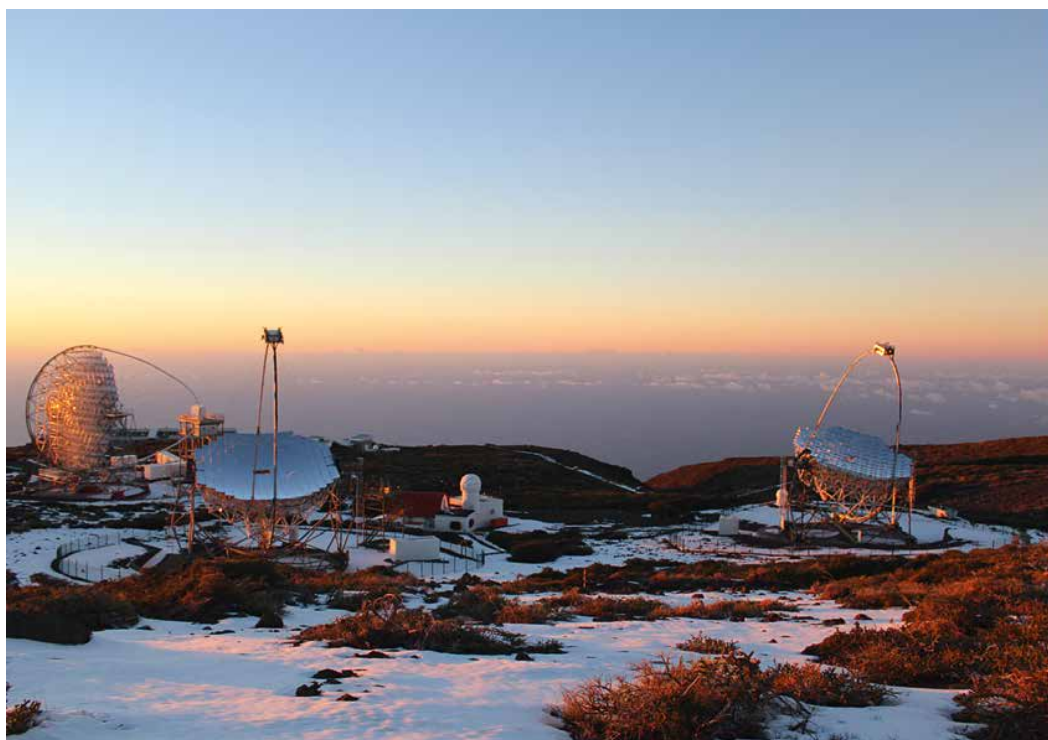
Eyes into space: the two MAGIC telescopes on the Roque de los Muchachos register particle showers in the Earth's atmosphere and use them to make indirect observations of gamma light from the depths of the universe.
