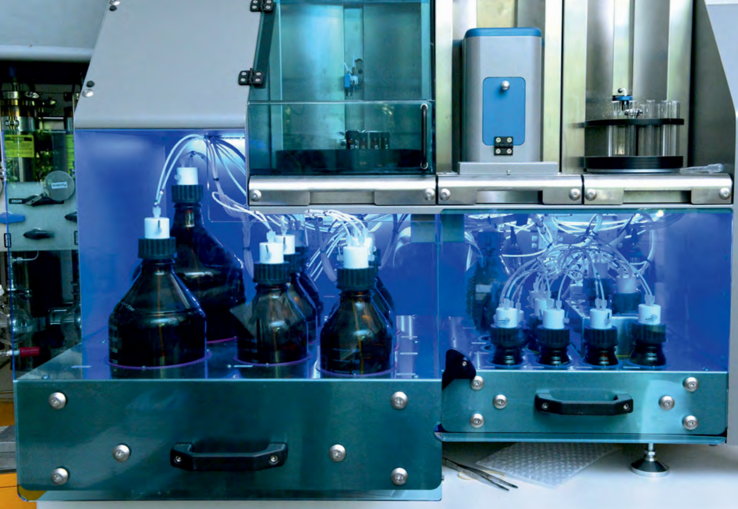
Automated sugar synthesis: the synthesizer brings the reactants together at the right time and in the right quantity. Seeberger commercialized this method at the Ancora Pharmaceuticals and GlycoUniverse companies.
