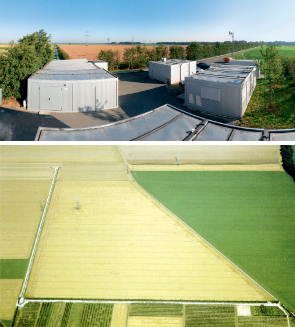
Field research: The GEO600 site in Ruthe, near Hannover. In the container-based offices and measuring stations (top) researchers analyze the data they obtain in the 600-meter-long interferometer arms (bottom). Under a protective cover hangs the vacuum tube in which the laser travels between the beam splitter and the end mirror (right).
